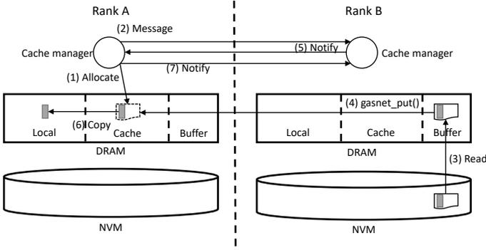
Fig. 2. Basic get operation of vGASNet
