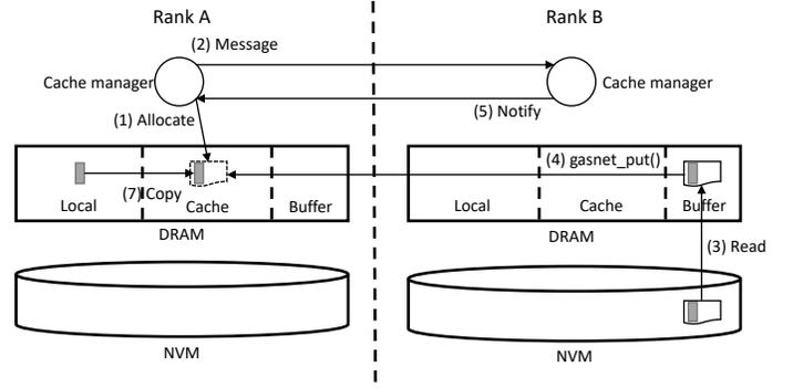
Fig. 4. Basic put operation of vGASNet
