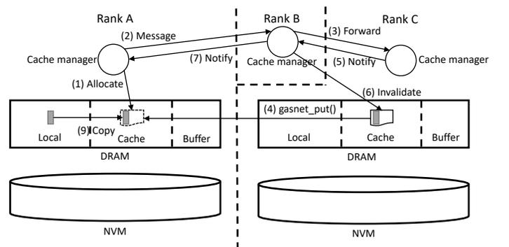
Fig. 5. Put operation of vGASNet with cooperative-caching
