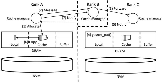
Fig. 3. Get operation of vGASNet with cooperative-caching
