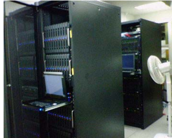
IBM/Appro Blade cluster Xeon x 2CPU x 200node SMP cluster
